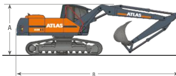
Adjustable boom 1.95 m (C21.41) and 3.83 m (C21.461)
