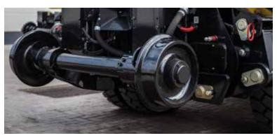
As option available: Friction Drive System available for 1404 ZW with track width 1000 and 1435 mm.
